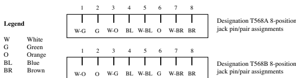
Eight-position jack pin assignments
